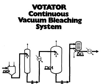
For the continuous bleaching of edible fats and oils • Excellent color reduction and scap removal • Low clay dosage. Low oil retention • Effective deaeration and dehydration. Effective oil-clay contact • Efficient utility usage. Minimum operator attention • Automatic control of process variables.
